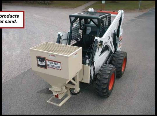
The Herd Salt/Sand Spreader is the Tool for Efficient Deicing. Ideal for Parking Lots and Walk-Ways, The model 750SSS couples the versatility of today's Skid Steers with the Durability that Herd is known for. Utilizing our unique agitator design, the Herd Salt/Sand Spreader is the most effective method of spreading any combination of sand (wet or dry), salt, and calcium chloride.
